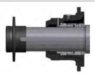
Seals type are interchangeable on the standard pump. Each solution was carefully engineered while taking into consideration all the operating conditions. As well as changing the sealing system, you can also install various types of mechanical seals based on the application.
