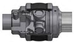
Joint protection: In the DHS or JHS series the joint rubber sleeve and clamp are protected from a particular device integrated inside the end of the auger feed screw. This characteristic is of considerable importance because it ensures the integrity of the joint in the case of pumping of abrasive substances or with solid blunt, without the needed to add expensive optional
