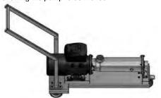
Modular Design: The RL Series is based on a modular concept in every single feature: hydraulic parts, casings, seals, stands, supports and drive shafts. Each component can be constructed in a number of variants without modifying the structure of the machine, thus maintaining standard replacement components.
