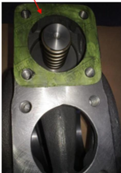
Fit the **tensor cap, number 8,** with the fixing bolts and fit the **tensor stud, number 9.**
