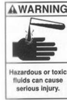
If pumping dangerous or toxic fluids, the system must be washed and decontaminated inside and outside before maintenance
