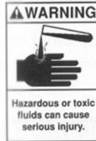
If hazardous fluids are pumped or toxic, the system must be washed and decontaminated, both inside as outside, before maintenance.
