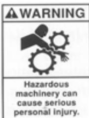
Serious injuries to persons, damage to property or death may be caused by operating the pump without the protections properly installed.
