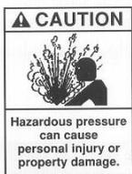
Snjury to persons or damage to property may be caused by if the system is not depressurised before undertaking maintenance on the pump.
