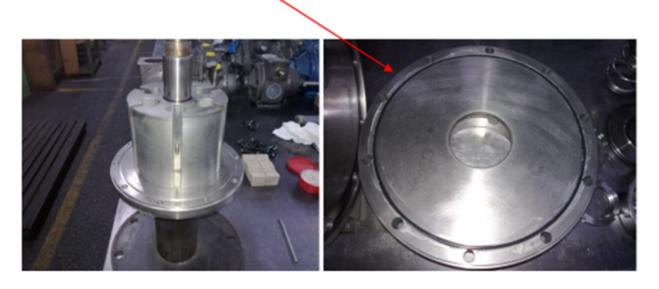
Before fitting the pump body, number 1, insert the with a little grease to prevent their falling.
