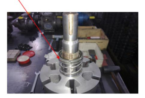
Carefully fit the **cover**, **number 2 D**, until it is seated on the face of the rotor, number 5.
