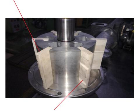
The vanes, number 6, must be fitted with the **channels** facing the pump's direction of rotation and with the rounded edge facing outwards on the rotor.
